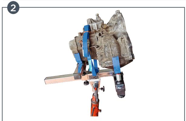
**7** - Move the rear crosspieces to the centre beam according to the length of the gearbox. Secure the front and rear arms against the gearbox.
