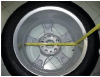
Figure F3.3.1. 1 Example of manual measuring of the external diameter (da2) of the wheel in the ALS1/ALS2 Programme Type
