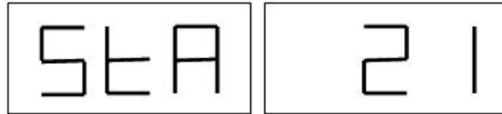
Fig. F8.1 View of the Static imbalance display enabled. The right display indicates the entity of the static imbalance.
