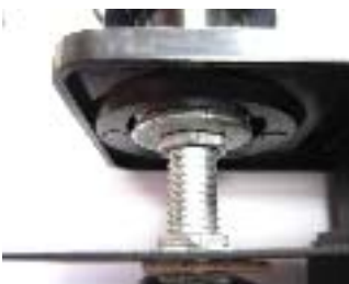
Nuts/Washers Installed Between L Bracket and Faceplate
