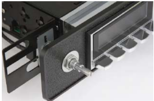
Figure 4 - Install Vehicle Specific Faceplate
