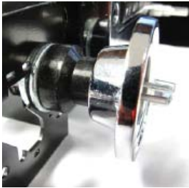
Figure 5 - Shaft Cover Installed
