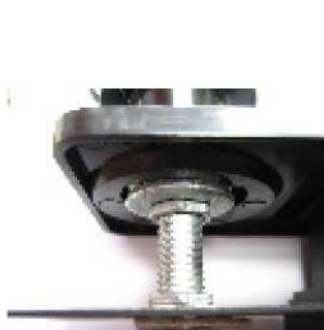
Nuts/washers installed between L bracket and faceplate
